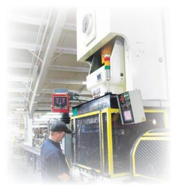
By knowing who needs to see it from where, it's easy to decide on the mounting and physical size of the unit. Small machines and work stations can use small stack tower lights. A small machine run by a single operator may use a smaller diameter & profile stack tower light. A longer process or assembly line where there may be multiple operators, QC technicians, or supervisors will need a stack light that is visible from a greater distance.
