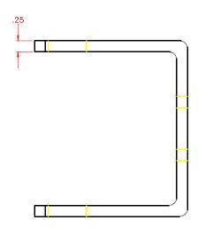
Material: Cold Rolled Steel. Plated
